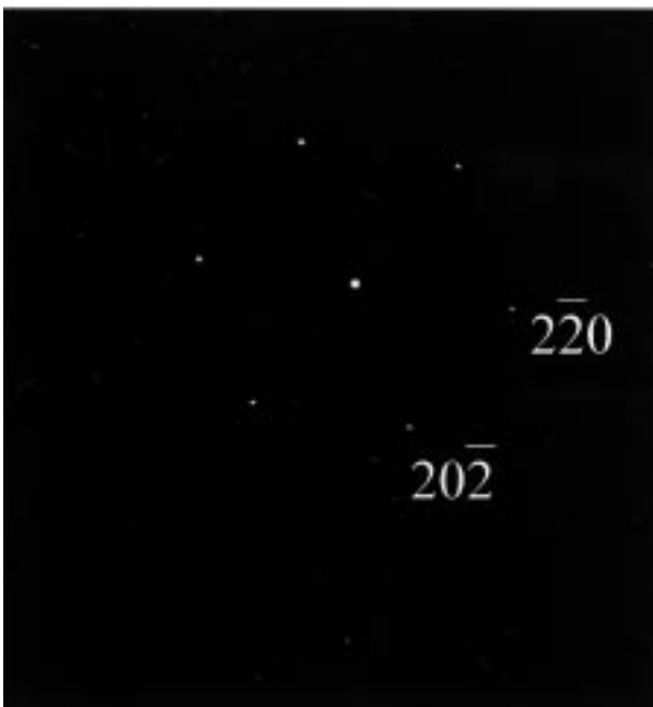
Figure 3 [1 1 1] zone patterns for each set of the tweed bands in as-cast Liberty. The bottom electron diffraction pattern can be obtained by a 120° counterclockwise rotation of the top electron diffraction pattern.
